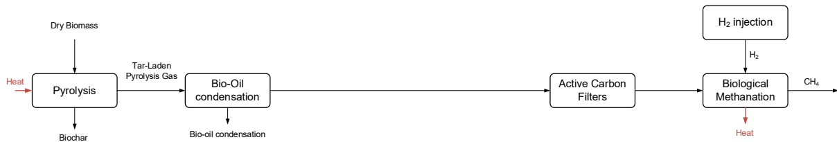
Figure 7 – Block diagram for the configuration bio-oil and methanation with H 2 addition
